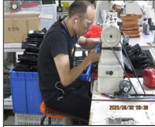
Photo of non-conformity NC Sewing machine missed belt guard.JPG
