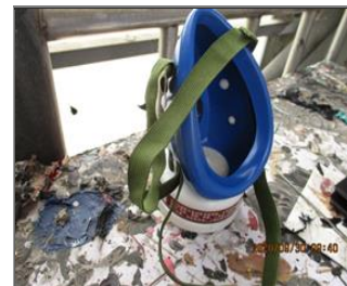
Photo of the personal protection equipments (if applicable) Mask for paint worker.JPG
